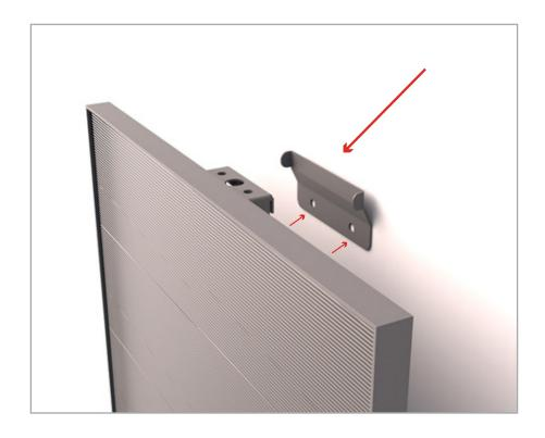
Notice the gap left for the hanging apparatus to mount on;
